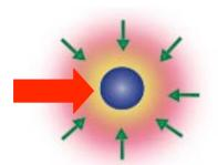
Direct drive illumination Laser beams rapidly heat the surface of the fuel capsule.
