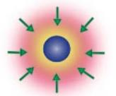
Direct drive illumination Laser beams rapidly heat the surface of the fuel capsule.
