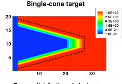
Energy distribution of electrons with 0.5<E<2.0MeV [/n<sub>c</sub>mc<sup>2</sup>],
