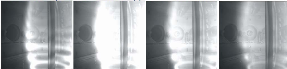
400 V bias: plasma streams appear to reconnect
