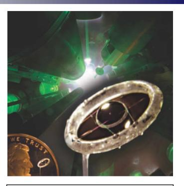
A Saturn target comprising a fusion-fuel containing capsule surrounded by a ring for achieving highly symmetric PDD implosions.
