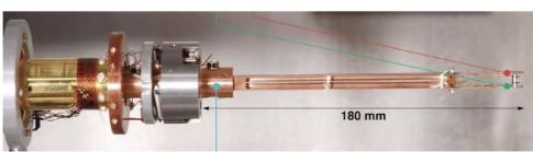
NIF cryo-system demo - 27 days of continuous operation with 1 mK target base stability
