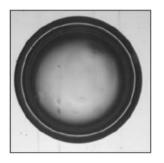
Demonstrated 1µm rms inner surface roughness DT ice layer
