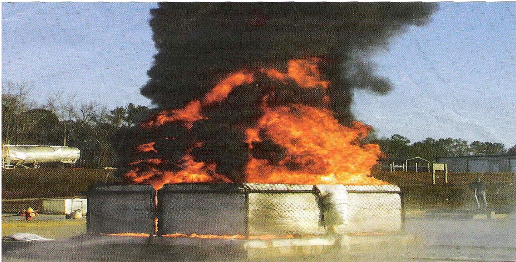
Savannah River's radioactive materials container, the 9977, underwent testing by fire to demonstrate its suitability for certification. (Photo: DOE)
