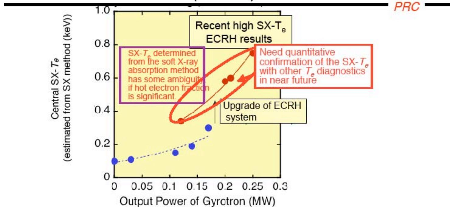
**No saturation of power scaling of SX- $T_e$**
