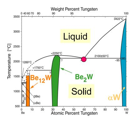
Melting point is reduced with increasing Be concentration:
