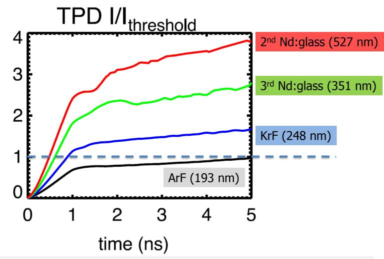
I\_threshold [10<sup>15</sup> W/cm<sup>2</sup>] = 8.06 \* Te[keV] \* 1/(laser\_wavelength[um]) \* 1/Ln [um] (Simon et al., Phys. Fluids 26, 3107 (1983).)
