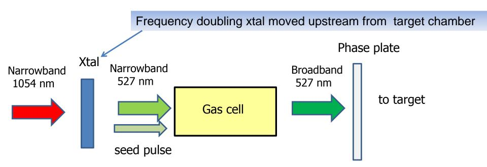
Green light → potential for substantially more energy on target for indirect drive Broad bandwidth → suppression of LPI and CBET in gas filled hohlraums
