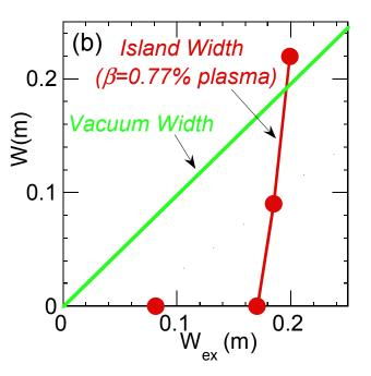
• Magnetic island existing in the vacuum field is healed, when the size of magnetic island is small (w<0.3a)
