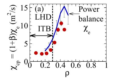
Significant reduction of thermal diffusivity inside the ITB is observed both in steady-state and transient transport analysis
