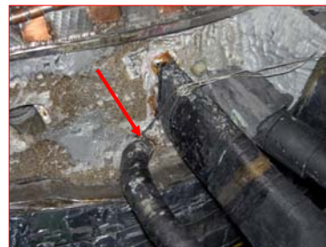
Cracks and cavities detected by Paschen tests
