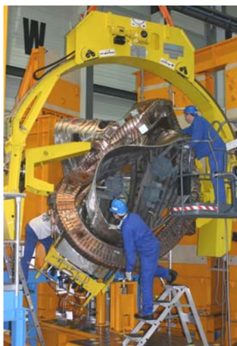
Threading of non-planar coil type 3 across the PV sector.
