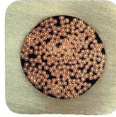
NbTi conductor with Al jacket
