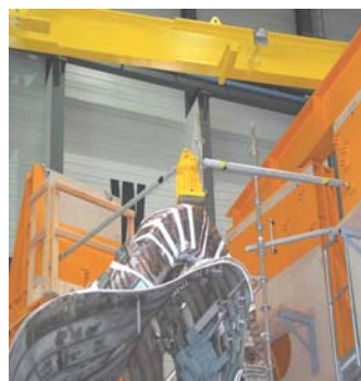
Non-planar coil type 3 fixed on top by adjustable poles.
