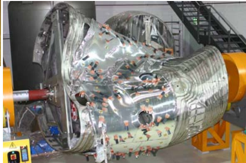
Thermal insulation on a vacuum vessel sector
