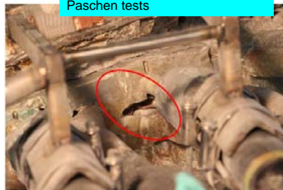
Cracks and cavities detected by Paschen tests
