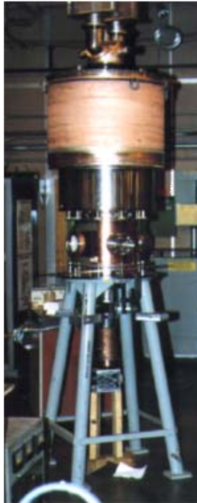
100 GHz Gyrotron Tube (1MW power in 1 second pulse) for Plasma Heating and Control
