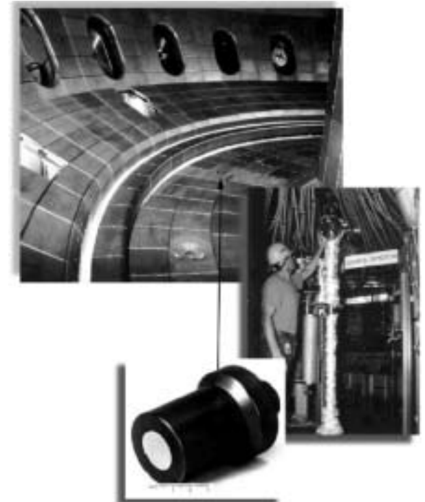
DiMES probe in DIII-D provides data on plasma material interactions
