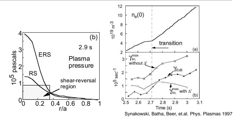
Internal transport barrier forms when the flow shearing rate  $\partial v_{\theta}/\partial r > \sim$  the linear growth rate  $\gamma_{lin}^{max}$  of the instabilities that usually drive the turbulence.
