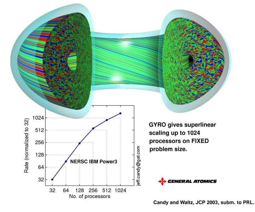
Comprehensive computer simulations being developed. Plasma Microturbulence Project movies & viz. at http://fusion.gat.com/theory/pmp Computer simulations recently enhanced to include all key effects believed important in core plasma turbulence (solving for particle distribution functions  $f(\vec{x}, v_{\parallel}, v_{\perp}, t)$  w/ full electron dynamics, electromagnetic fluctuations, sheared profiles).
