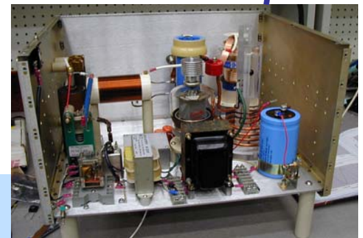
500 \mu s, 20kW, ~ 10 MHz Compact RF oscillator
