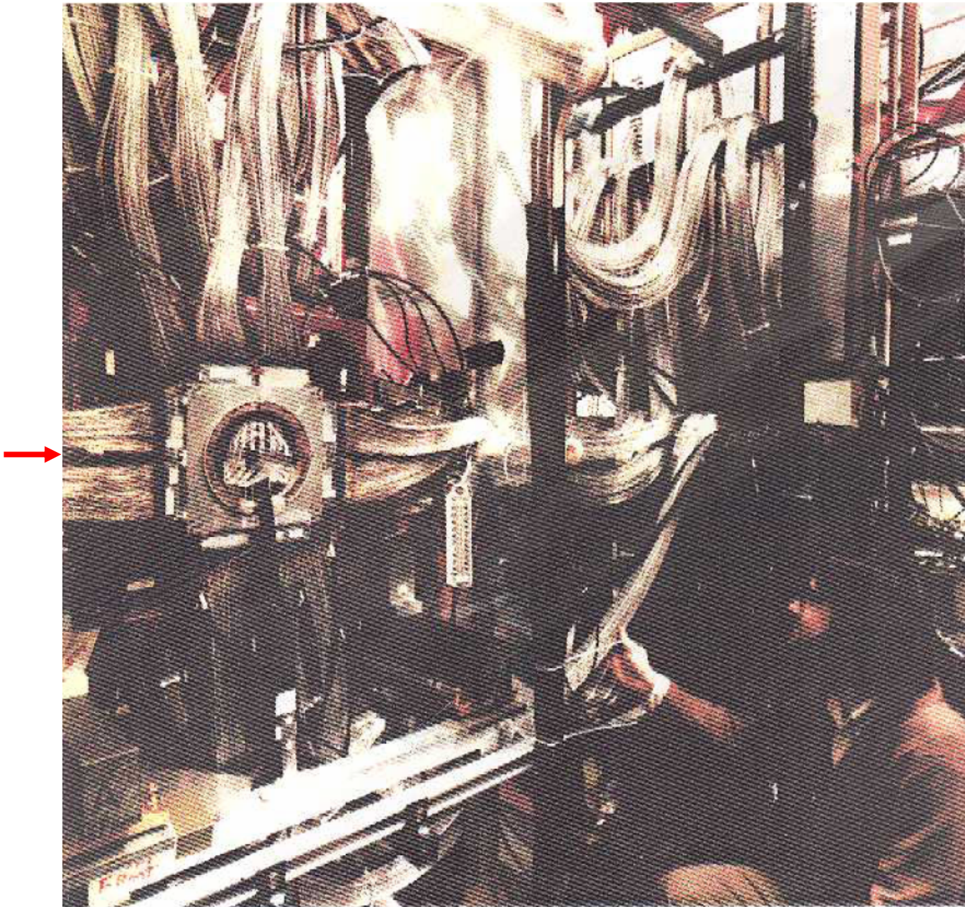
Paul Karchin in front of a silicon telescope (the rest of the photograph: fanouts and cables). (Fermilab; 1985, 9 planes, 5 cm x 5 cm)
