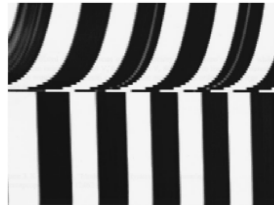
FIG. 4. Experimental image. A line-pattern; with 3.0 \mu\text{m} period is scanned upwards. At the center of the image the scan offset was changed from -80 to 0 V while the SPM continued scanning. The curvature is typically related to "creep" but also contains time-independent transition.
