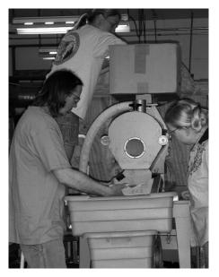
The seed is placed in the feed pan hopper positioned at the top of the machine. A larger 25 liter feed hopper pan is available for large seed amounts. As the seed falls through the feeding funnel, the small metal paddles located at its mouth push seed into the shaft that houses the rotating blades. A vacuum cleaner hose attached to an opening above the mantle jacket removes fine dust. A powerful shop-vac works very well. Small seed and debris fall through the mantle into a collection pan.
