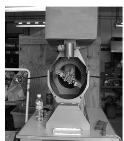
Extensive training and supervision is not necessary to learn how to operate the machine; however, a two person operation is recommended - one person to stand on the ladder and dump seed into the hopper: the other person to observe the seed expulsion so the bins do not overflow.
