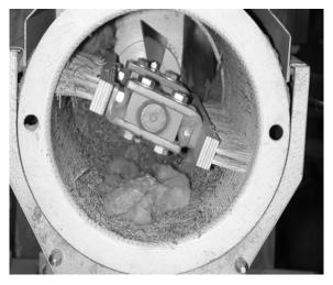
(Michx.)Nash which was conditioned at speed 8 and the seed was run through the machine twice. Sometimes the seed does not completely separate from its other parts during the first run so more passes are necessary.
