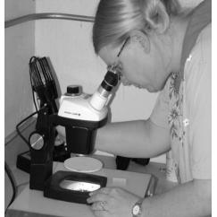
Britton, are hard to see with the naked eye, therefore, magnifying equipment is needed to distinguish seed from chaff. Magnifying lamps, dissecting scopes, and microscopes are most commonly used for viewing seed. Magnifiers allow the operator to view the condition of the seed, and evaluate the conditioning operation. More passes through the brush machine or additional equipment may be needed to remove the
