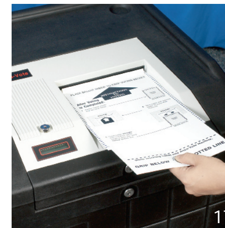
When a voter completes their ballot, the ballot should be inserted into the AccuVote unit. The ballot is tallied and pulled into the ballot box.
