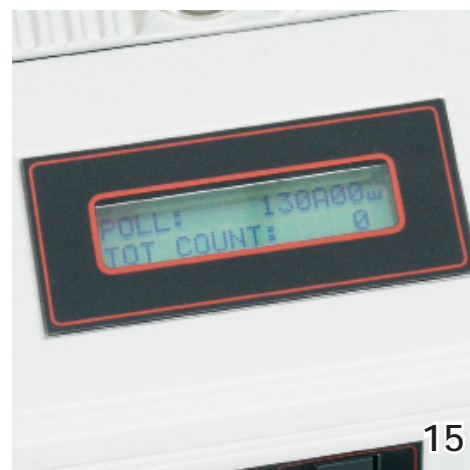
Verify the LCD display on the AccuVote Unit shows the precinct or poll number and that the public counter (TOT COUNT) is at "0."
