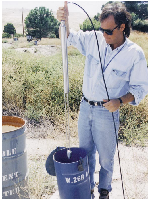
Figure 20. LLNL is using the colloidal borescope to aid in well placement and to evaluate the progress of ground water remediation.
