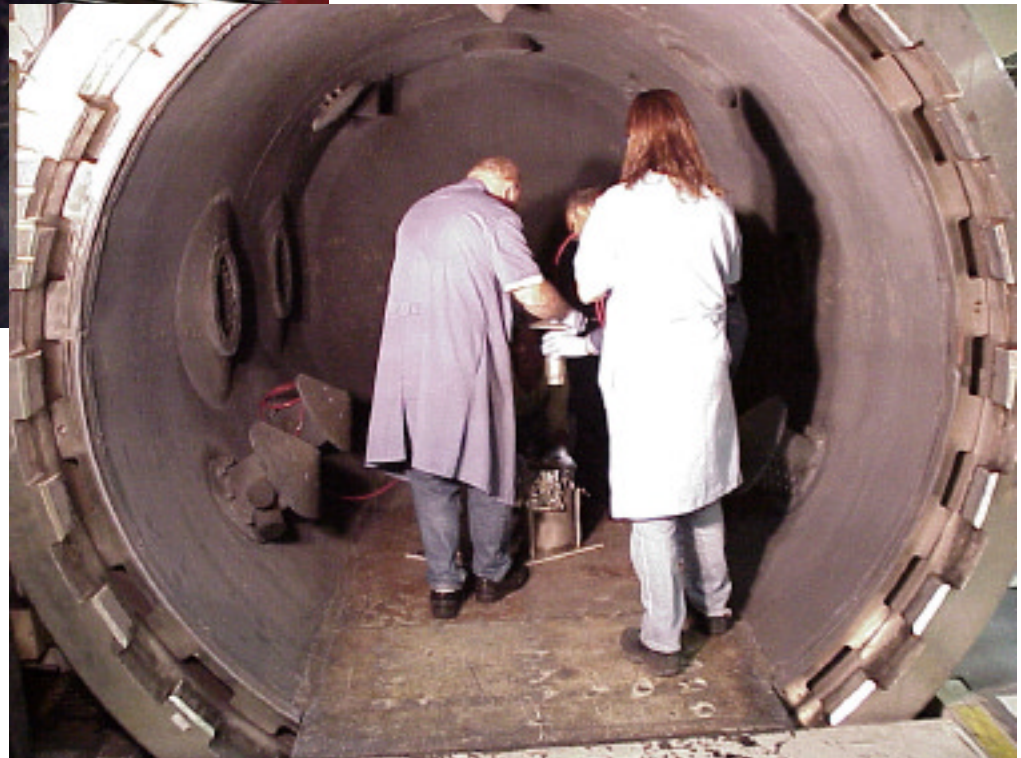
Photo 9. Filled inner assembly installed into outer vessel.
