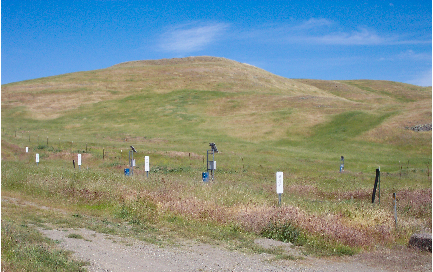
Infiltration trench used for the discharge of treated effluent from the Pit 7-Source ground water treatment system and piezometers
