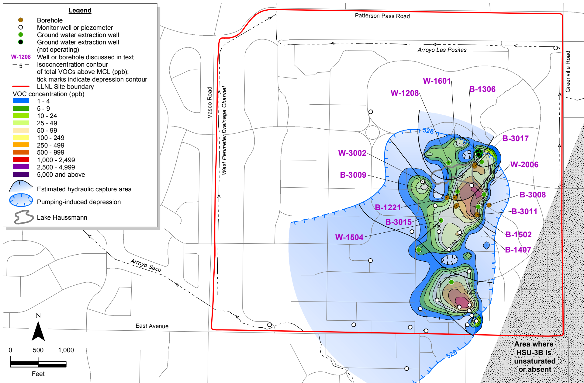
Figure 12. Isoconcentration contour map of total VOCs above MCLs from 42 wells completed within HSU-3B, third quarter 2014 (or the next most recent data), and supplemented with soil chemistry data from 112 borehole locations.
