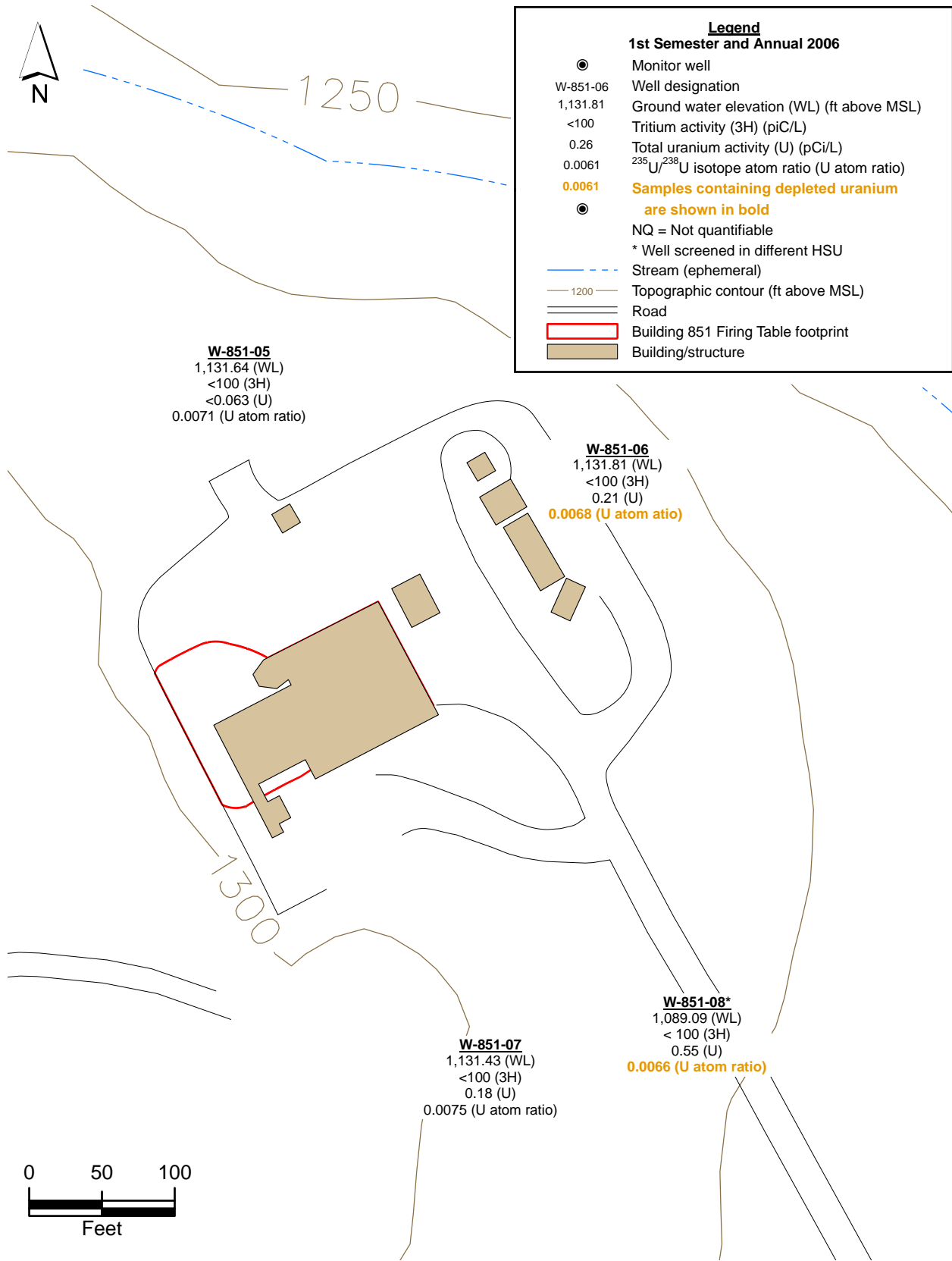
Figure 2.8-4. Building 851 Firing Table site map showing monitor well locations, ground water elevations, tritium activities and uranium activities, and 235 U/ 238 U isotope atom ratios in the Tmss HSU.
