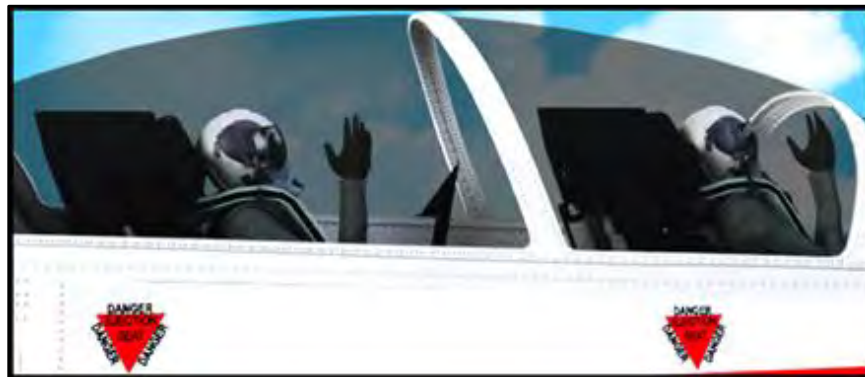
Figure 4-6 Kiss Off Signal
