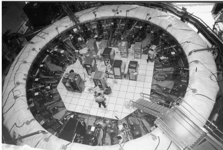
Fig. 21. A photograph from above of the muon ( g-2 ) storage ring. The four quadrupole pulser units are located in the middle of the ring, with one unit being worked on.
