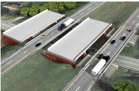
Step 1: Construct superstructure next to existing bridges
