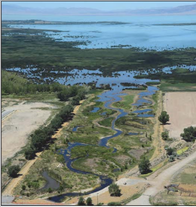
Reconstruction and restoration of the lower Hobbble Creek channel where it enters Utah Lake was completed in late summer 2008. The restored area allows delivery of recommended supplemental flows through lower Hobbble Creek and to Utah Lake.
