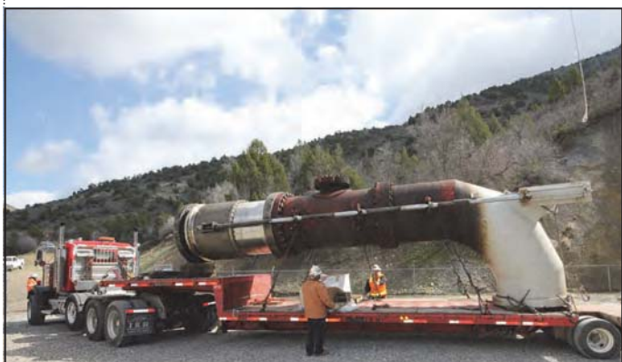
Sixth Water Flow Control Structure Damaged Sleeve Valve
