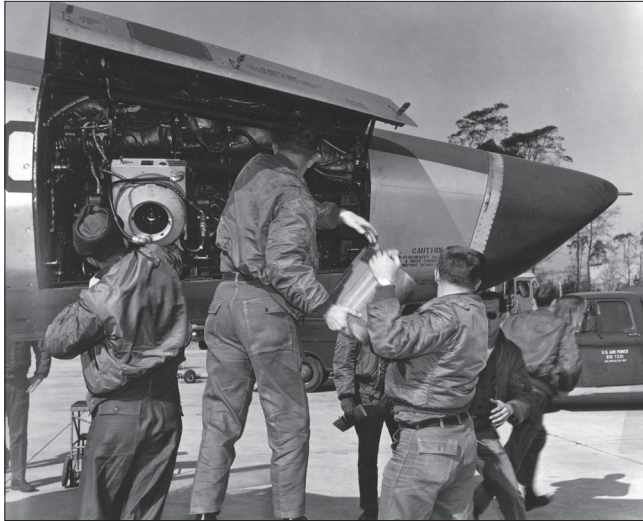
Figure 2. The film arrives at the end of a reconnaissance mission, to be rushed to the base film processing unit. (Photo courtesy of the National Museum of the Air Force)
