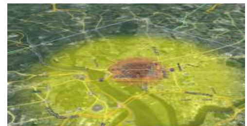
Light Damage Zone Outer boundary may be defined by the prevalence of broken windows 1. Zone extends from ~1 mile up to ~3 miles (10kT Example) 2. Damage NOT caused by dynamic (wind-like) pressure, but the "shockwave peak free field overpressure" 3. Damage not just to windows, but other larger flat (and weak) features 4. Mostly superficial wounds from flying glass and debris
