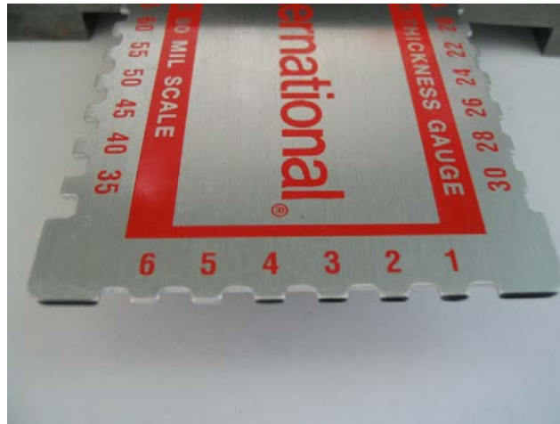
Figure 5. WFT Gauge Showing a Reading of 4-5 Mil.
