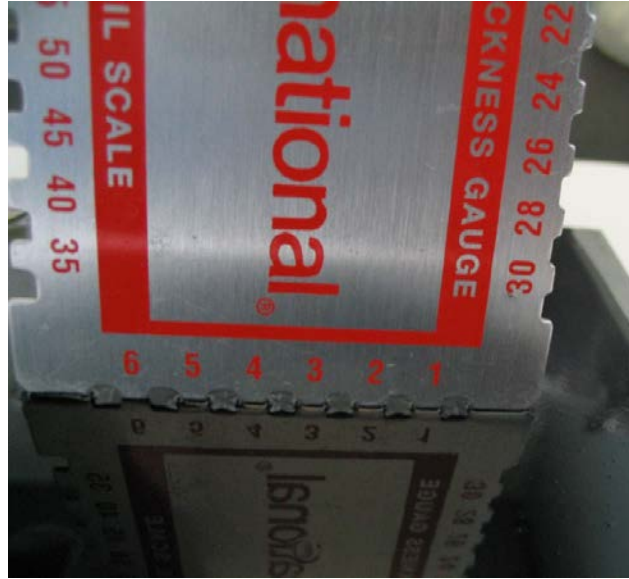
Figure 4. WFT Gauge Positioned in Wet Paint Film.
