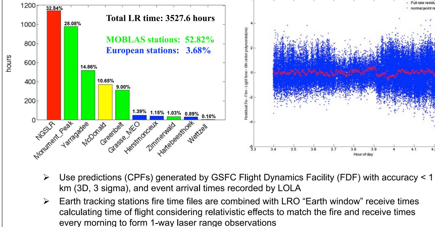
> One way LR precision:  $10 \sim 50$  cm for full rate, and  $2 \sim 5$  cm for normal points
