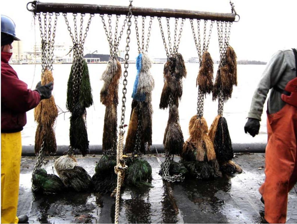
Figure 3. The Vessel-Submerged Oil Recovery System (V-SORS) that is being used to search for and recover submerged mobile oil on the river bottom. The chains keep the sorbents along the bottom. The oil readily adheres to the snares underwater.
