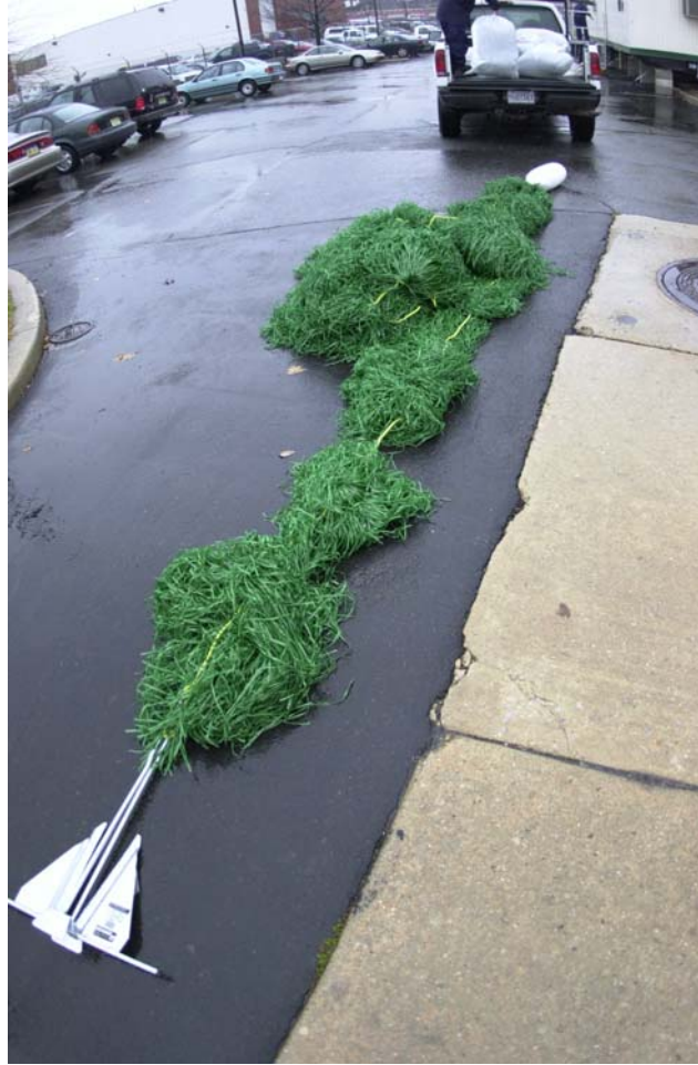
Figure 2. The snare sampler system consists of an anchor, a 50 ft string of snare on a rope, and a float. The samplers are inspected regularly and the percent oil coverage at different intervals is recorded. Most of the time, the heaviest oiling is on the bottom several feet.
