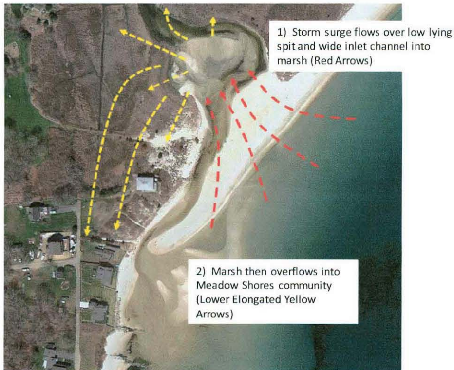
Figure 12: Storm surge flooding via marsh
