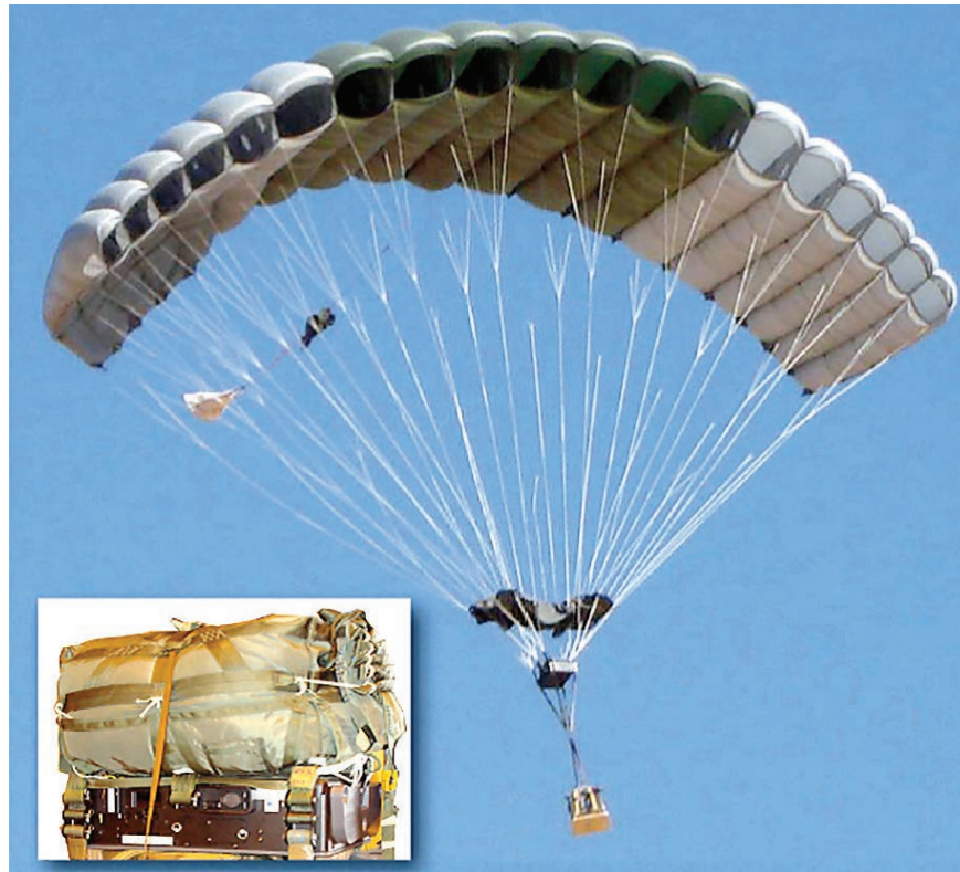
The Joint Precision Airdrop System, or JPADS, is intended to provide increased tactical maneuverability and enable a sustainment capability to support total Army, multi-service, and multi-national ground forces. The JPADS Air Vehicles are a family of high altitude systems offering weight capabilities of 500, 2,400 and 10,000 pounds.
