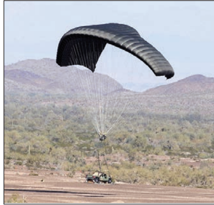
ABOVE: The Joint Precision Airdrop System has various weight capabilities. Shown here is a demonstration of the 10,000 pound capability. RIGHT: The air vehicle uses a 2,000 pound capability to deliver its cargo. Engineers at Picatinny Arsenal are applying their expertise in software reliability so that the advanced precision airdrop system can perform reliably under a variety of conditions.
