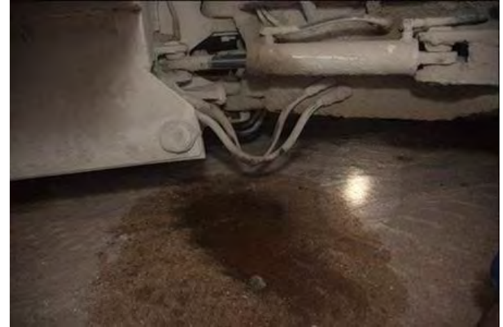
Hydraulic Leak under Sister Vehicle
