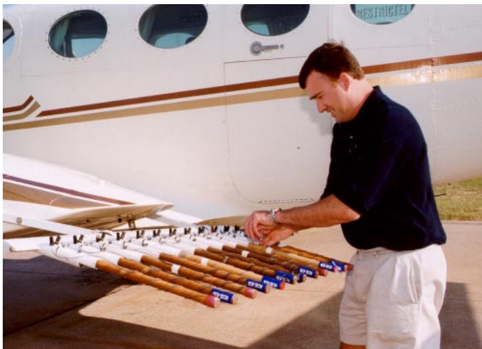
Tim Sedlock, Project Meteorologist for the Oklahoma Weather Modification Program, adjusts burn-in-place flares on one of two aircraft stationed at Oklahoma City's Wiley Post Airport.
