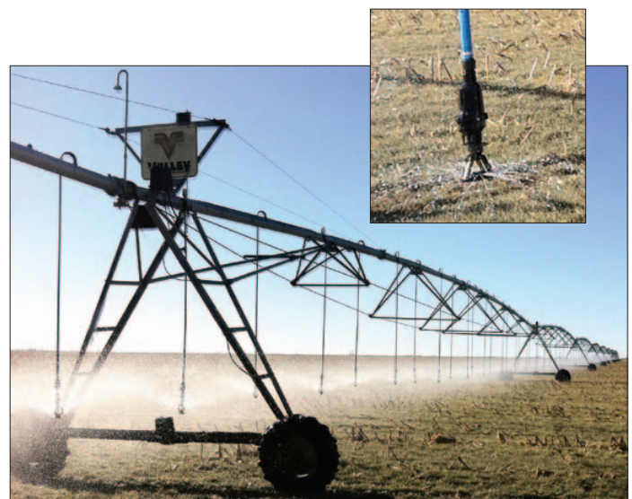
Center-pivot irrigation systems retrofitted with low-impact nozzles (see inset) positioned just above the crop, such as on this farm near Guymon, significantly reduce evaporative losses.
