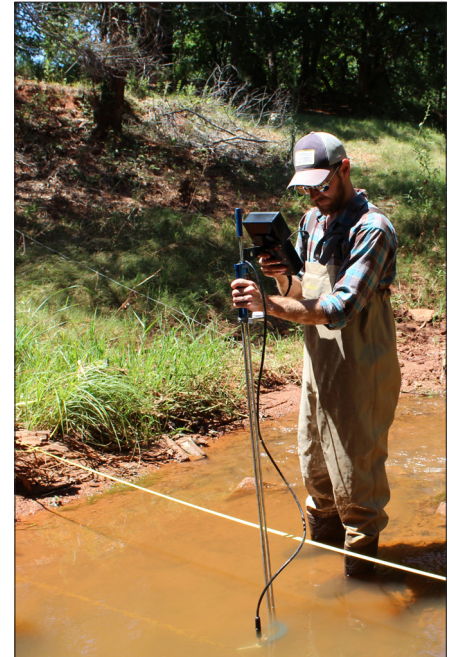
OWRB Geologist Kyle Spears measures streamflow in Oak Creek near Canute using a FlowTracker instrument as part of the Elk City Sandstone aquifer study. Streamflow measurements are an important component for estimating the amount of baseflow contribution, which can help derive important aquifer properties. The Elk City is one of eleven aquifers currently under investigation by the OWRB.
