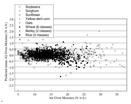
Figure 2. Predicted moisture measurement error for 15 grain types and 3 crop years with the unified moisture algorithm. (Funk, 2001)
