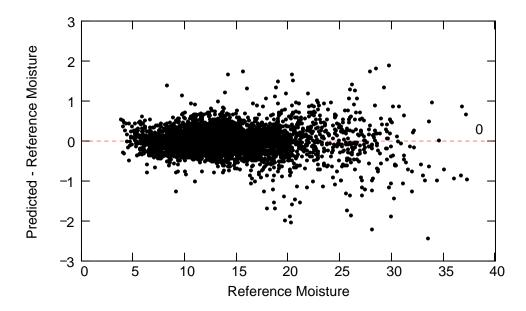
Figure 5. Performance of the Unified Moisture Algorithm (predicted minus reference moisture) for 5,141 samples representing 53 types of U.S. cereal grains, oilseeds, pulses, and processed rices for the 1998-2002 crop years.
