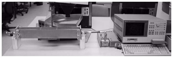
Figure 1. Transmission line test cell and HP-4291A RF Material/Impedance Analyzer
