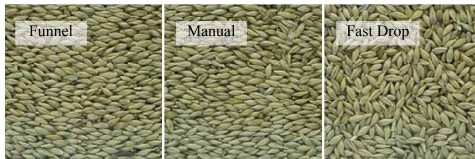
Fig. 6: Side view of transparent test cell (barley) loaded by funnel loading, slow pouring, and fast drop.
