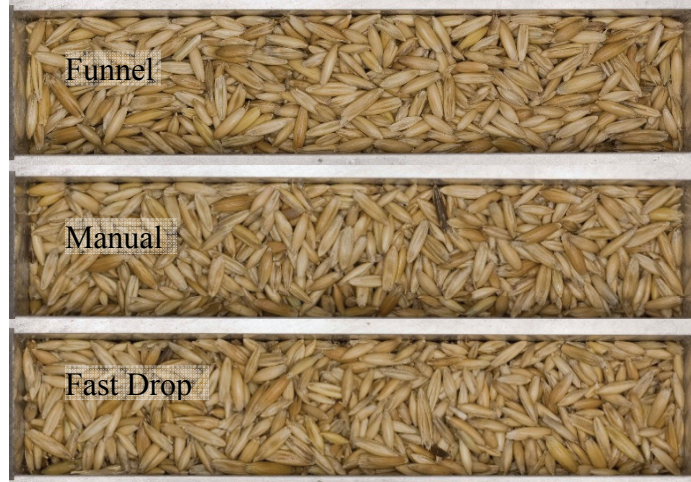
Fig. 7: Top views of (half of) test cell with oats loaded by funnel loading, slow pouring, and fast-drop.
