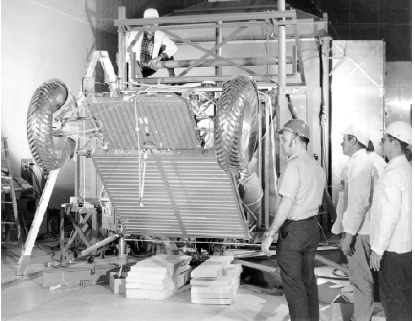
The rear wheels and chassis are ready for operation during deployment tests at Boeing's Kent, Washington facility.
