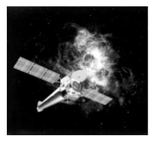
50,162 pounds and measured 45.3 feet long by 64 feet wide with its solar arrays deployed.
