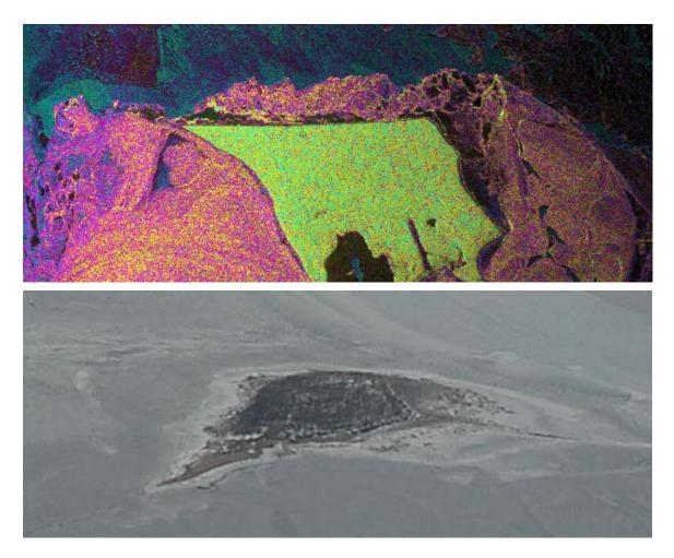
**Figure 8:** Images of ice surrounding Chambers Island in Green Bay, Lake Michigan: (a) Top panel is and L-band AIRSAR image for an ice area in Green Bay with color proportional to the ratio of the HH and VV polarimetric channels, and (b) bottom panel is an aerial photograph of the same location. Note that the look angles and azimuth orientations are different between the two images.
