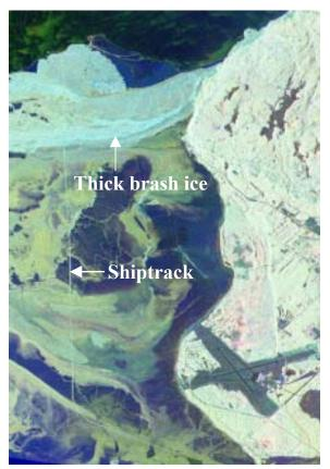
**Figure 4:** Zoomed-in SAR image revealing the US Coast Guard Mackinaw ship track encountering thick brash ice in the Whitefish Bay.
